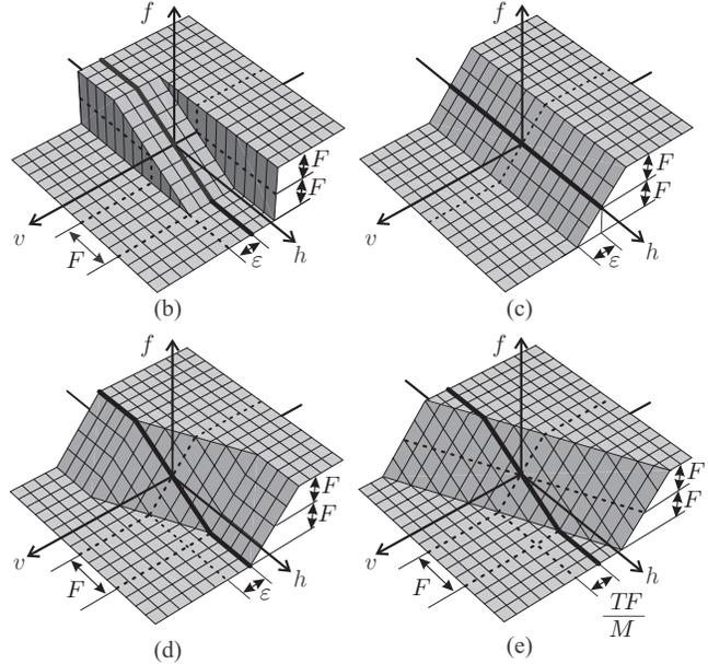
Fig. 3. Discontinuous friction models: (a) Coulomb friction model. (b) Karnopp's model [7], defined by (5) and (3), (c) viscosity approximation [14], defined by (6), (d) Quinn's model [8], defined by (7), and (e) the proposed discontinuous model, defined by (13). The thick black lines represent the value of  $f$  at  $v = 0$ . As  $\varepsilon \rightarrow 0$  or  $T \rightarrow 0$ , (b), (d), and (e) converge to (a).
